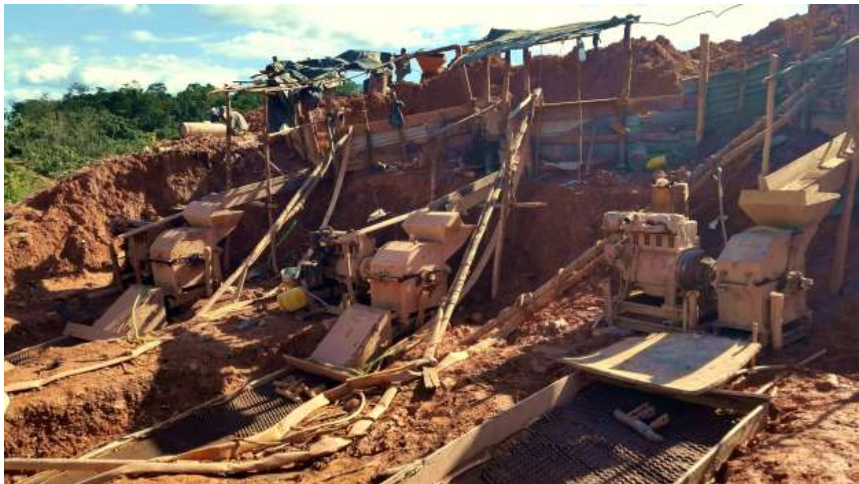
Figure 11. Crusher operation with three crushers in a line up
