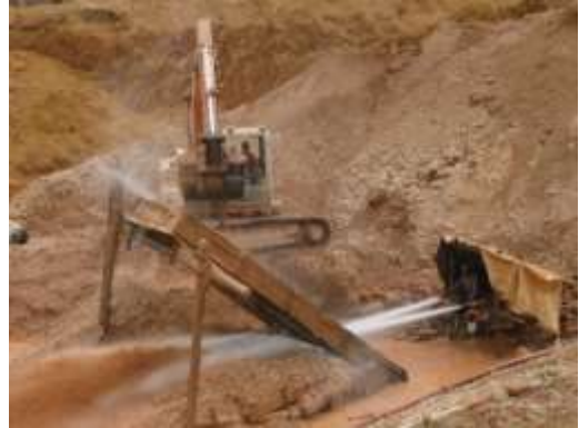
Figure 9. Use of a screen in hydraulic mining
