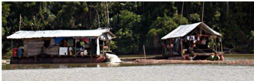
Figure 13. Two mining rafts ( pondos ), depositing their tailings in the river, this creating sand banks
