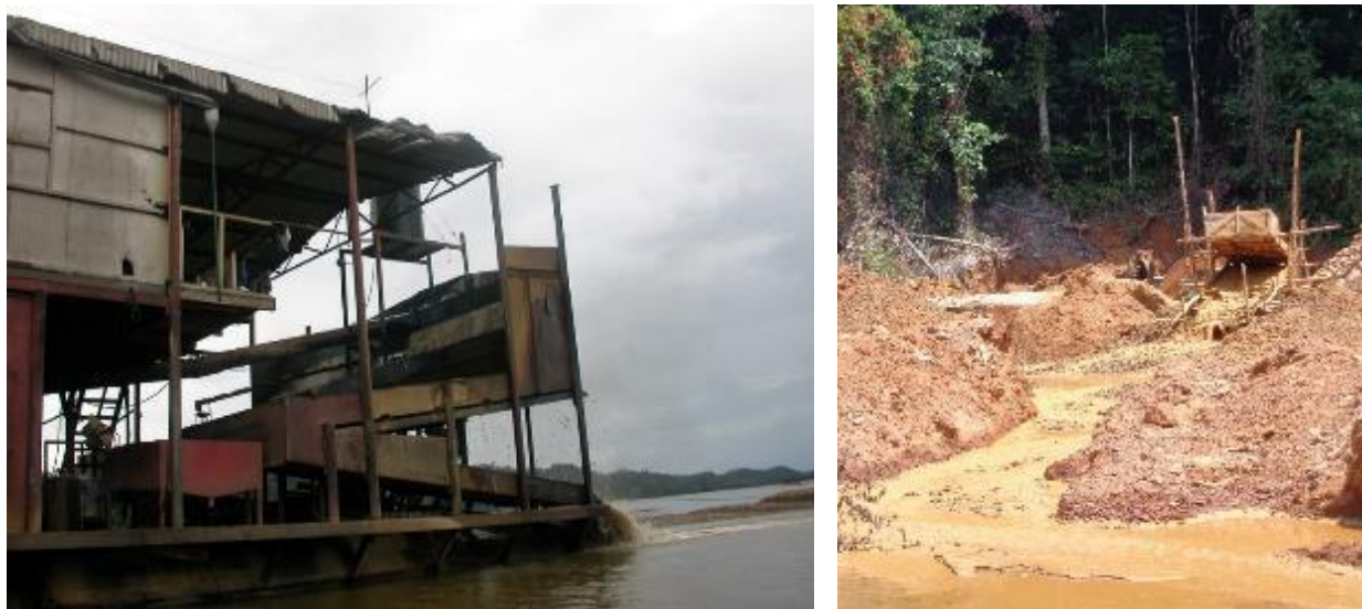
Figure 12. Water based mining from a raft (left), and land based hydraulic mining (right); in neither one of these cases are the sediments contained.
