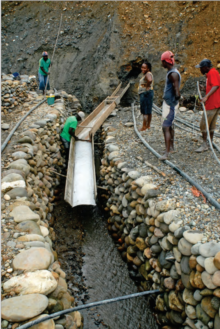
Artisanal mining method performed by Afro-Colombian communities where sands are washed utilizing water pressure. Ponds, gravity and occasionally small water pumps are utilized for creating pressure. Photograph by Oro Verde.
